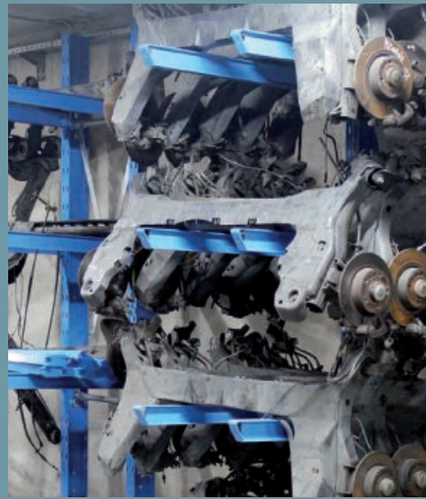
Storage facility of vehicle axles in cantilever racks. The distance between the columns is variable and the storage tiers are adjustable in their height.
