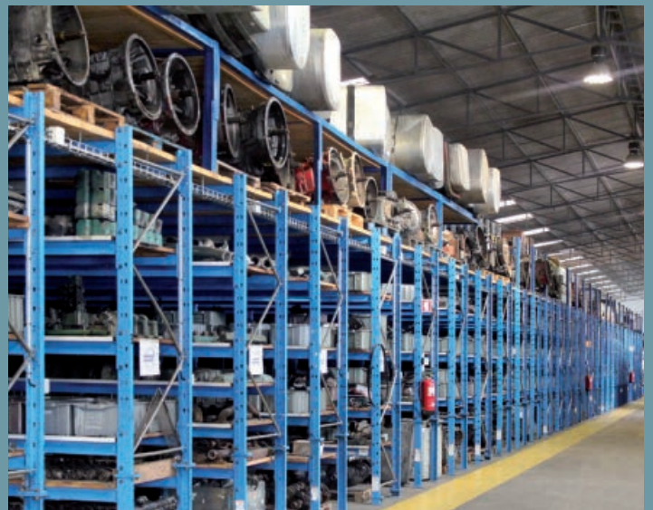
Combination of robust pallet racks for the storage of spare parts or small items while using the top level as an additional storage area for transmissions or bulky components.
