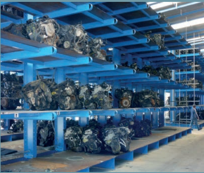
Storage of motors in robust cantilever racks. Through the use of arm-bridges a variety of different sizes can be stored in one level.
