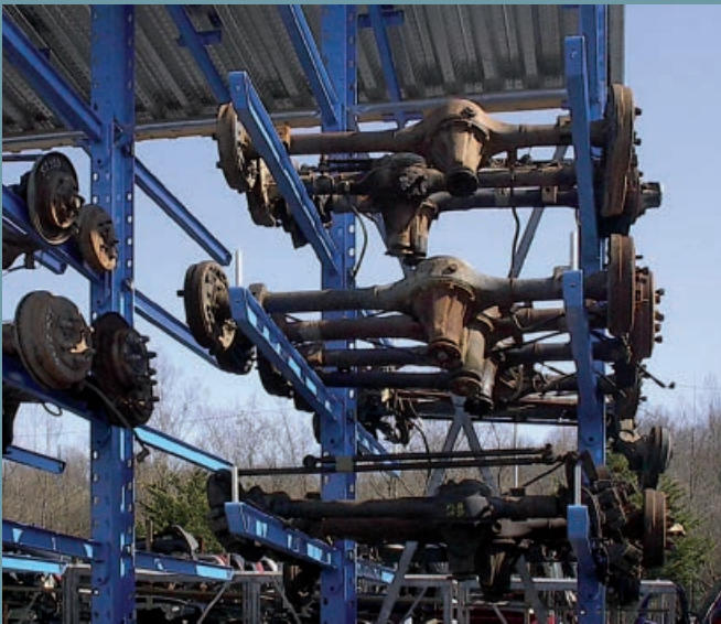
Several heavy axles stored well-organized in one level behind each other. This allows quick retrieval of the correct product and simple handling.
