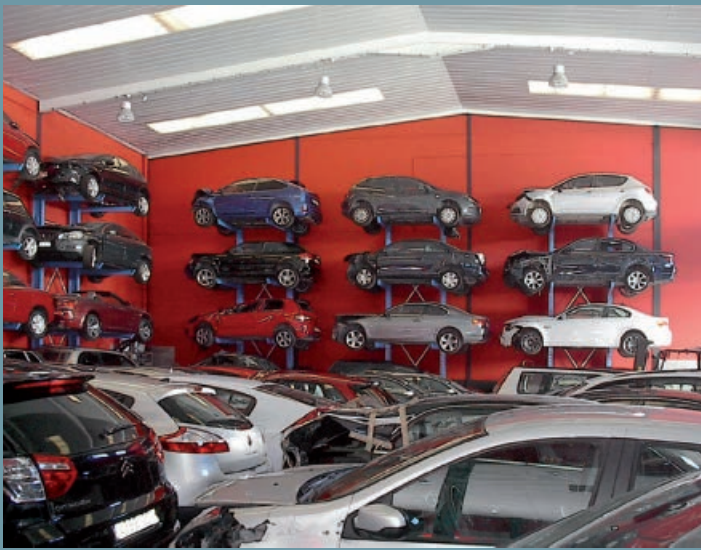
Clearly arranged storage of several vehicles on top of each other. Utilisation of the existing ceiling height and wall area.
